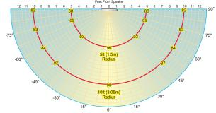
Measured at 2 watts setting in anechoic chamber
